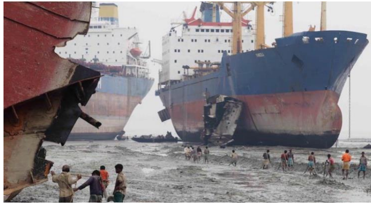
Fig 3: A Typical Picture of Beaching Method
