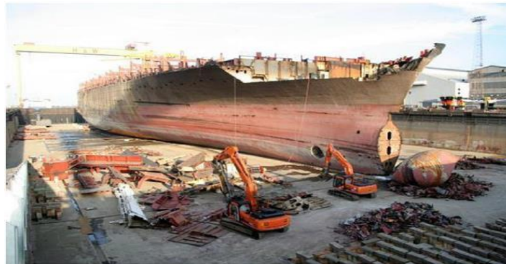
Fig 4: Ship dismantling in dry-docks in Belfast, Northern Ireland.
