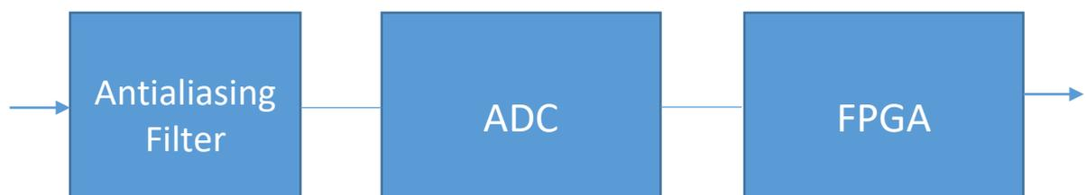
Figure 2.4: Digital partial discharge detection meter
