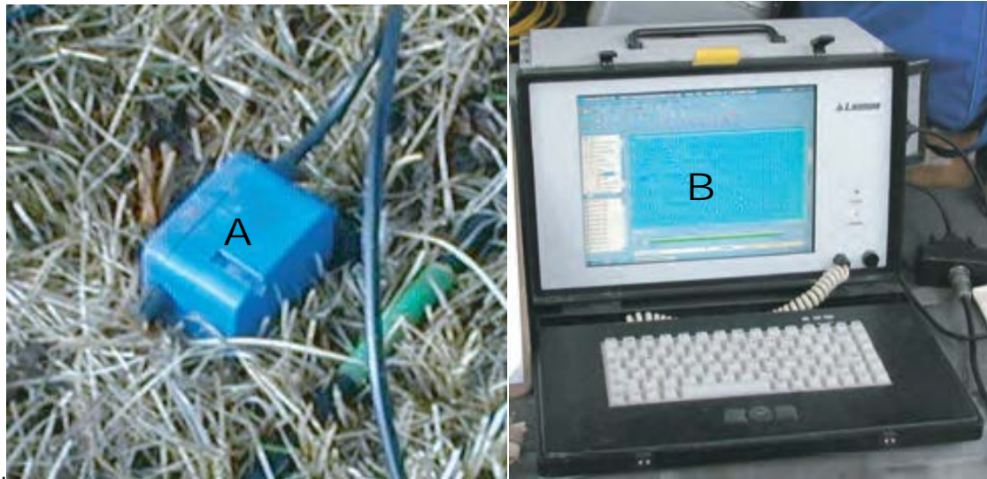
Figure 3.4: Apparatus used for S-wave seismic refraction profiling. A, Geophone used to detect the S-wave. B, Seismograph used to record the time-varying voltages generated by the geophones.
