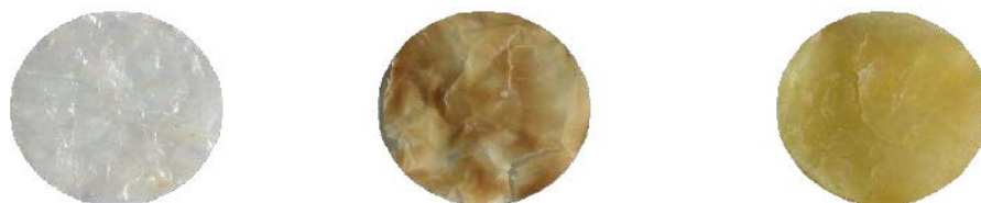
Figure 1. Bioplastic made from chitosan from fish scales (Source: Aziz et al 2017)
