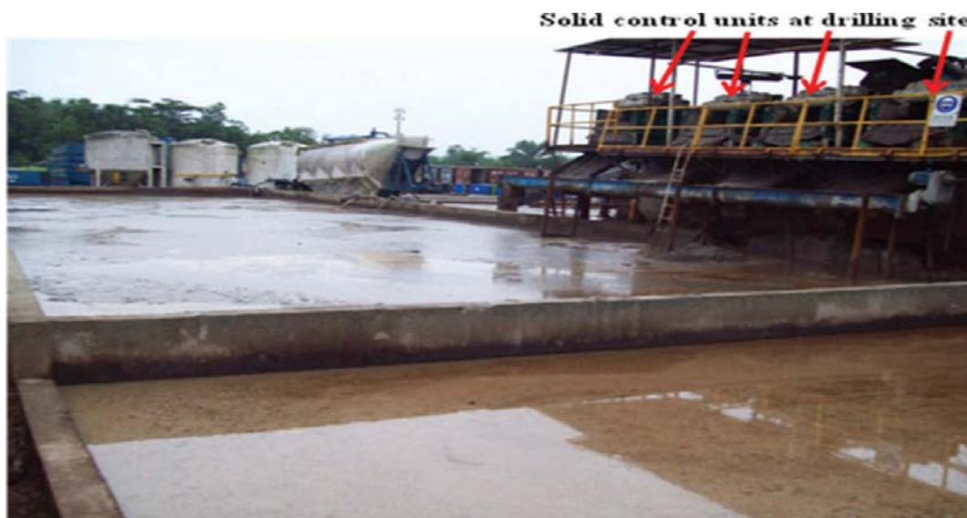
Figure 1 – Solid control unit in X field located in Niger Delta Nigeria (Onwuka et al. 2018)
