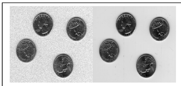
Fig 1.6:- (a) Poisson Noise (b) De-noised Image.
