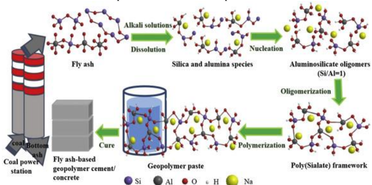
Figure: 2 The schematic drawings showing the process from fly ash to fly ash-based geopolymer cement/concrete
