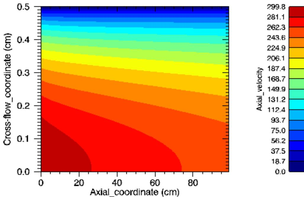
Figure 6. 9 Temperature and velocity distribution in axial direction for inlet flow of BP in equilibrium conditions (Axial coordinate vs Velocity distribution for 0.10 MPa)
