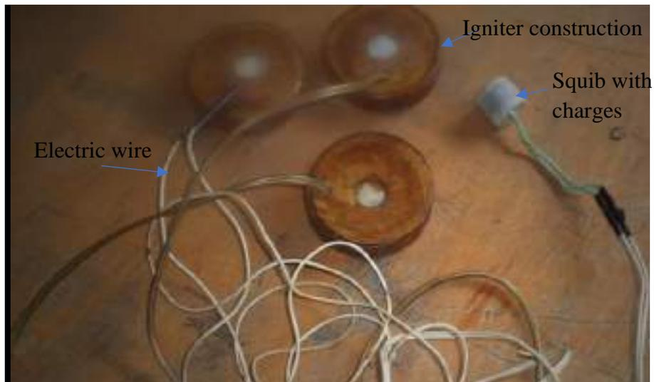
Figure 4.9 Design and construction of pyrotechnic igniter for particular SRM (Photo)
