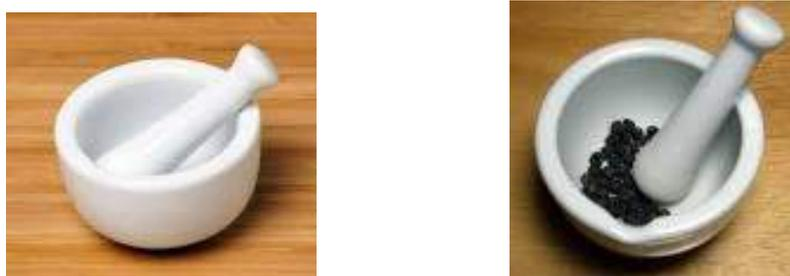
Figure 5.2 A set of mortar and pestle for grinding the chemical compositions
