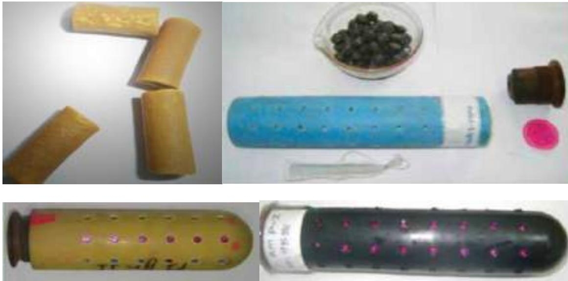
Figure 4.13 Multi perforated ignition charge of high energy material
