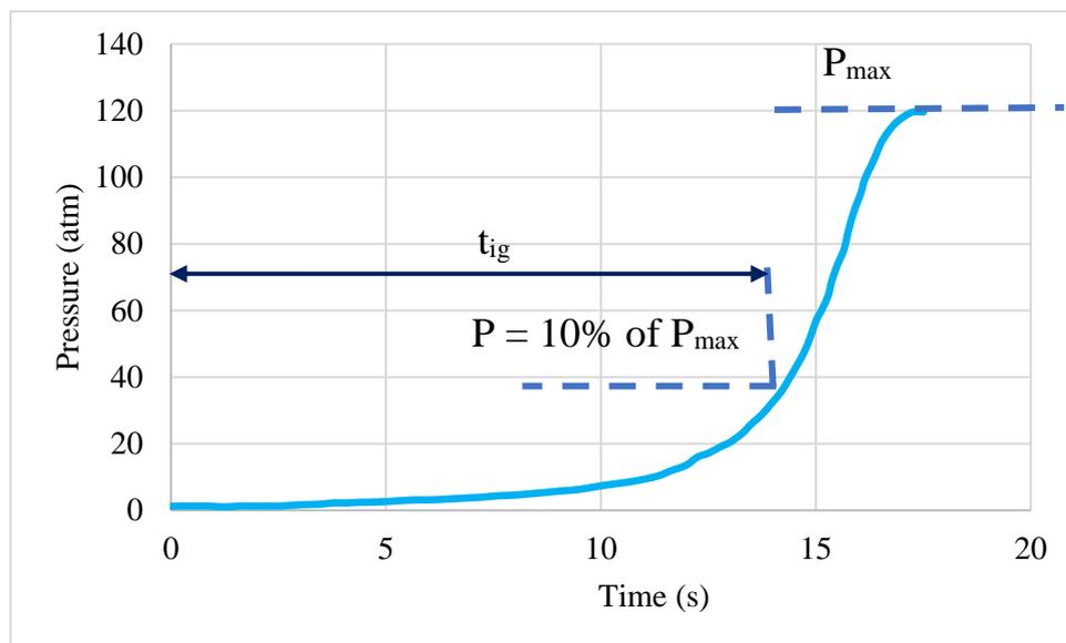
Figure 3.4 Pressure (P) versus ignition time ( $t_{ig}$ ) graph
