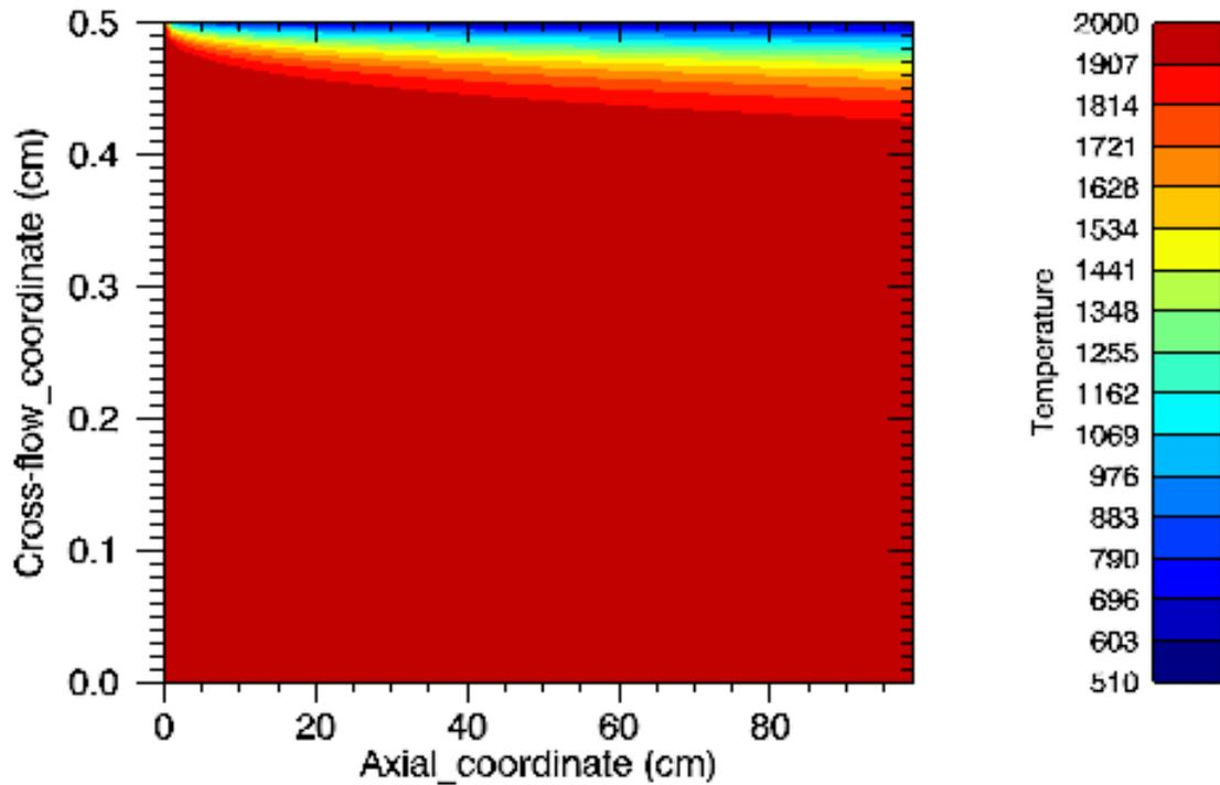
Figure 6. 10 Temperature and velocity distribution in axial direction for inlet flow of BP in equilibrium conditions (Axial coordinate vs temperature distribution for 5.00 MPa)
