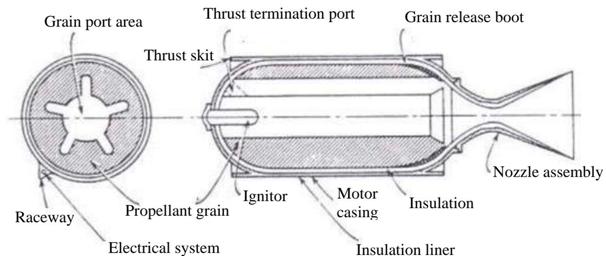
Figure 2.2 Generic SRM components and its cross-sectional view
