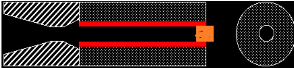
Figure 6.7 The energy flow from igniter to a cylindrical channel of propellant in SRM
