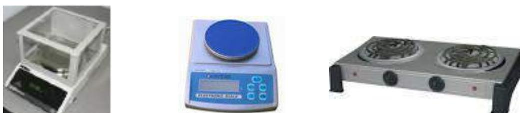
A) lab electronic balance      B) Electronic Balance      C) Electric stove
