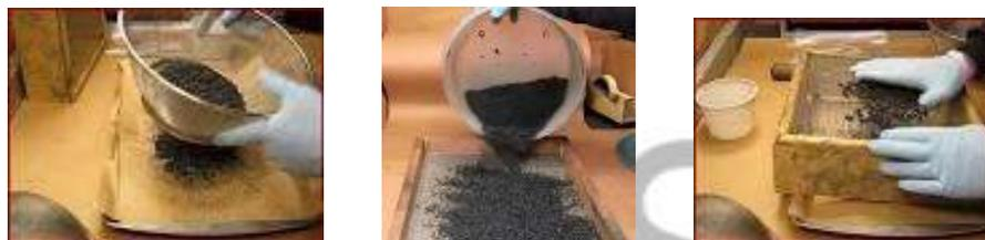
Figure 5.15 Crushing and sieving the powder to required grain size
