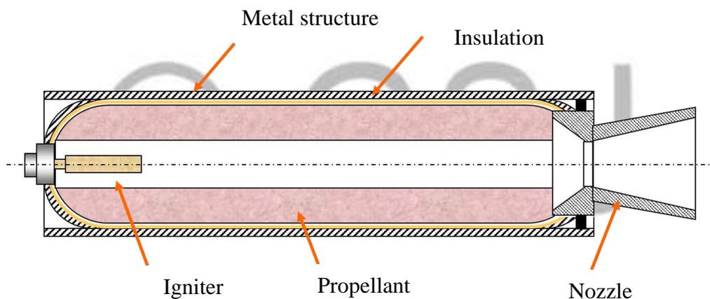
(a) Sectional view of rocket motor and its components
