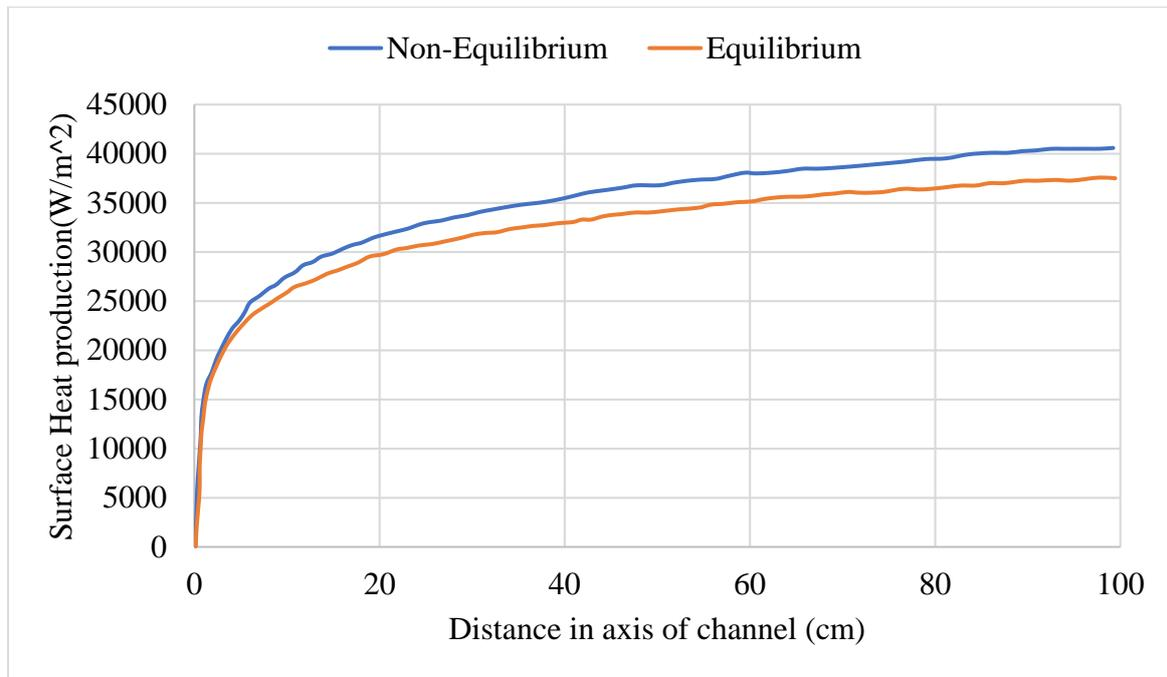
Figure 6.16 Estimated rates of surface heating for inlet flow for an inlet temperature of 2,000<sup>0</sup>K, and inlet pressure 0.10 MPa
