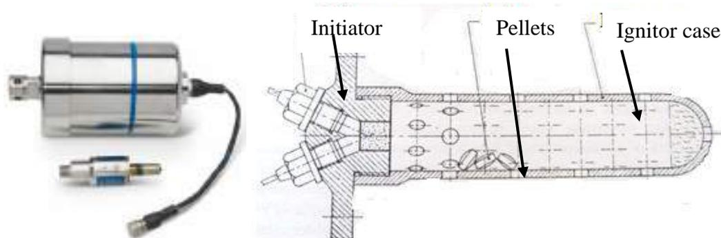
Figure 2.4 Pyrotechnic igniter
