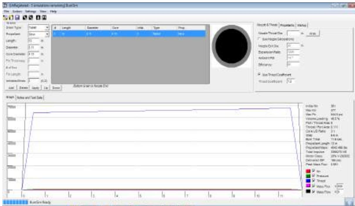
Figure 6. 2 SRM thrust simulation using BurnSim rocket internal ballistic performance simulation software for Tablet grain of slow burning propellant
