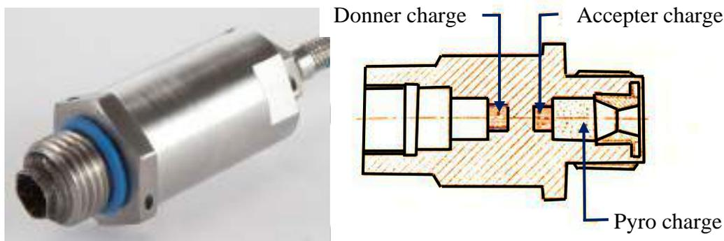
Figure 4.7 Through bulk-head initiator
