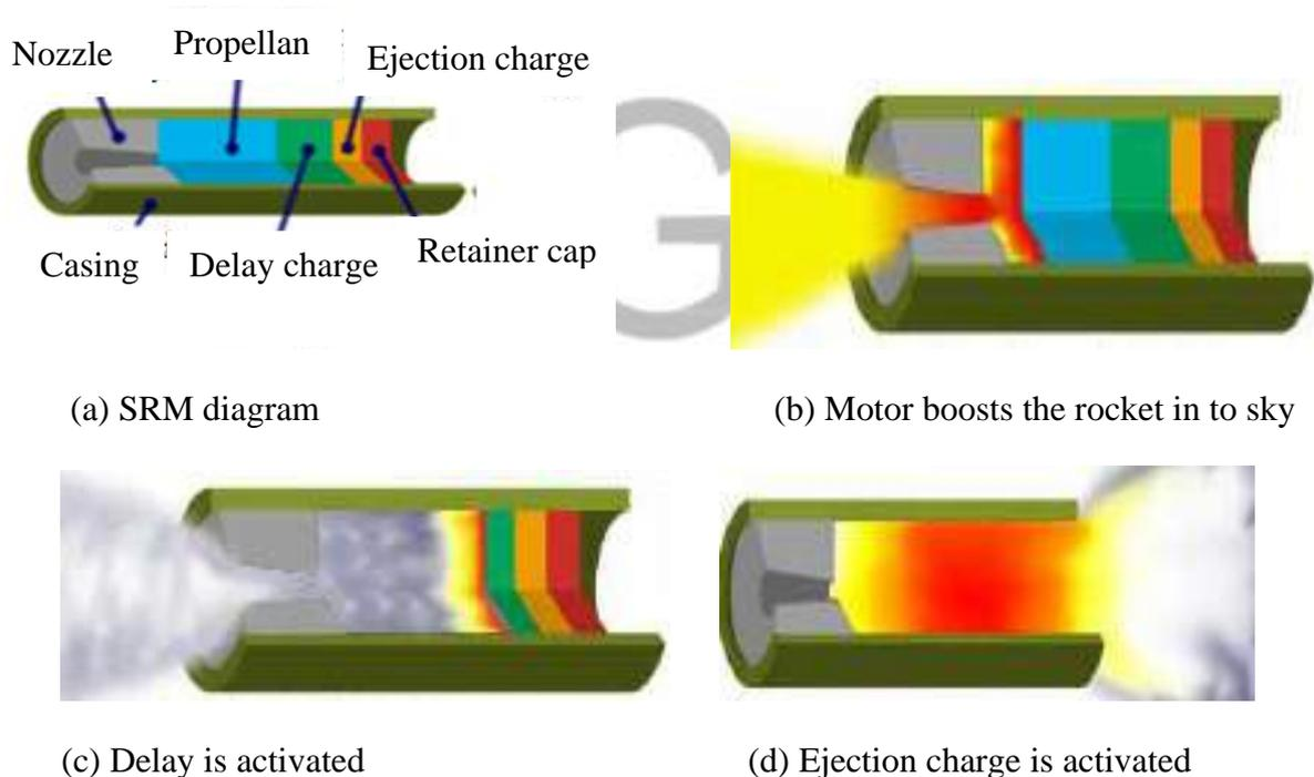
Figure 3.1 The diagram illustrates the working principle of
