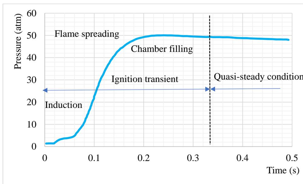
Figure 4.2 The ignition transient intervals of SRM
