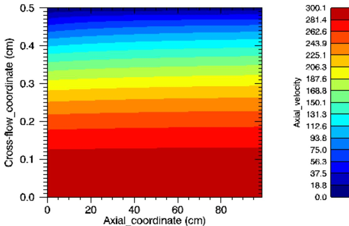
Figure 6.15 Temperature and velocity distribution in axial direction for inlet flow of BP in non-equilibrium conditions (Axial coordinate vs Axial velocity distribution for 5.00 MPa)
