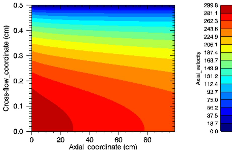
Figure 6. 13 Temperature and velocity distribution in axial direction for inlet flow of BP in non-equilibrium conditions (Axial coordinate vs Axial velocity distribution for 0.10 MPa)
