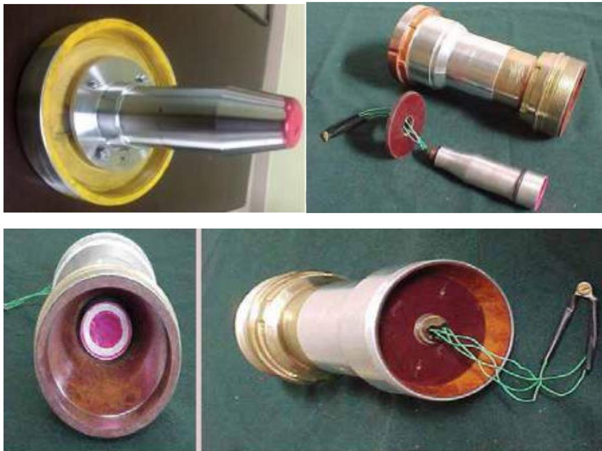
Figure 4.10 Alternative assembly of pyrotechnic igniter in SRM (Photograph)
