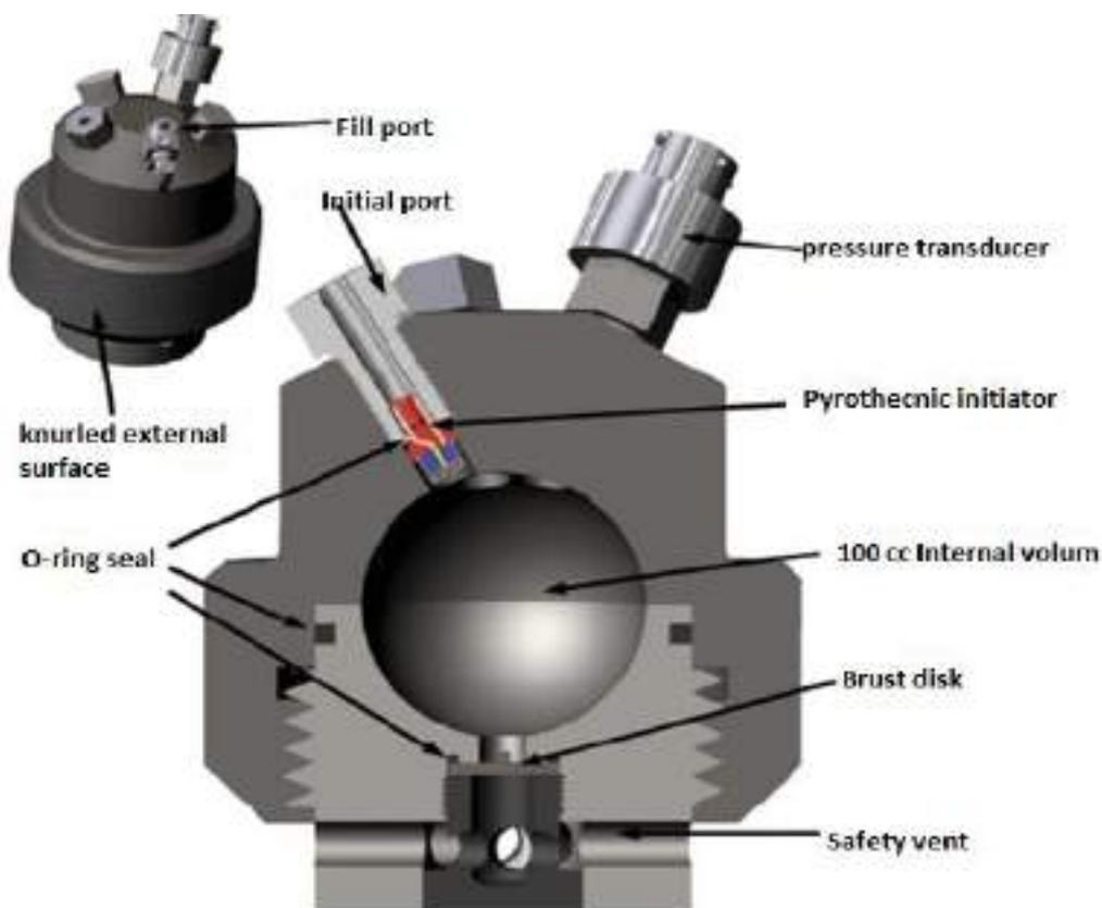
Figure 5.18 The ballistic test fixture for testing ignition charge or BP performance
