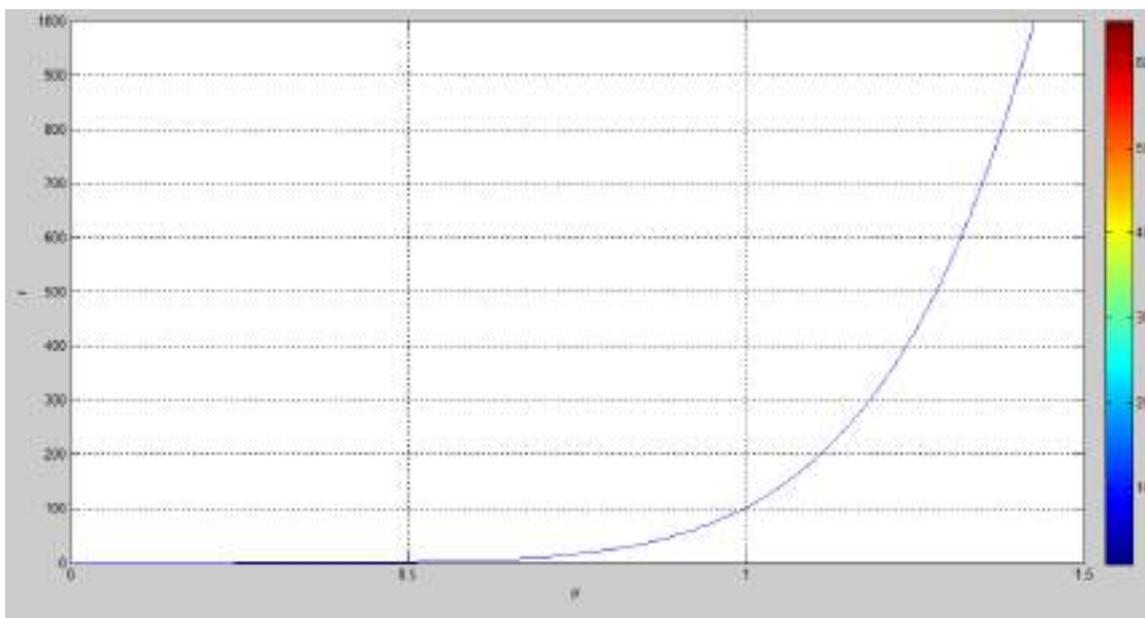
Figure 3.3 MATLAB simulation for combustion chamber pressure (Pc) versus burning rate (rb) for particular black powder ignition charge.
