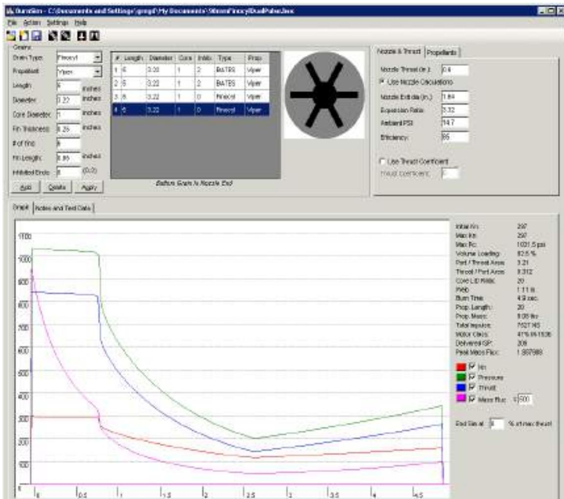
Figure 6. 1 Rocket performance simulation using BurnSim for 6point star Finocyl grain of past burning propellant type
