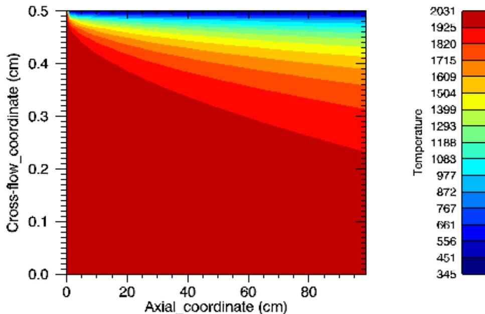
Figure 6. 12 Temperature and velocity distribution in axial direction for inlet flow of BP in non-equilibrium conditions (Axial coordinate vs temperature distribution for 0.10 MPa)
