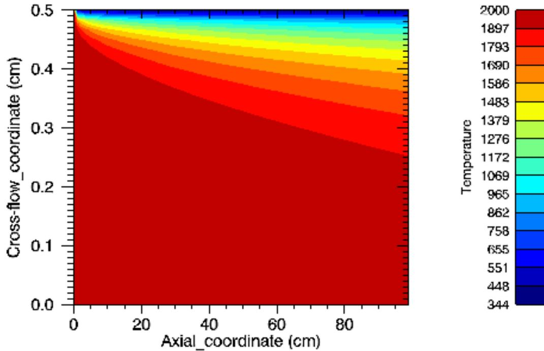
Figure 6. 8 Temperature and velocity distribution in axial direction for inlet flow of BP in equilibrium conditions (Axial coordinate vs temperature distribution for 0.10 MPa)
