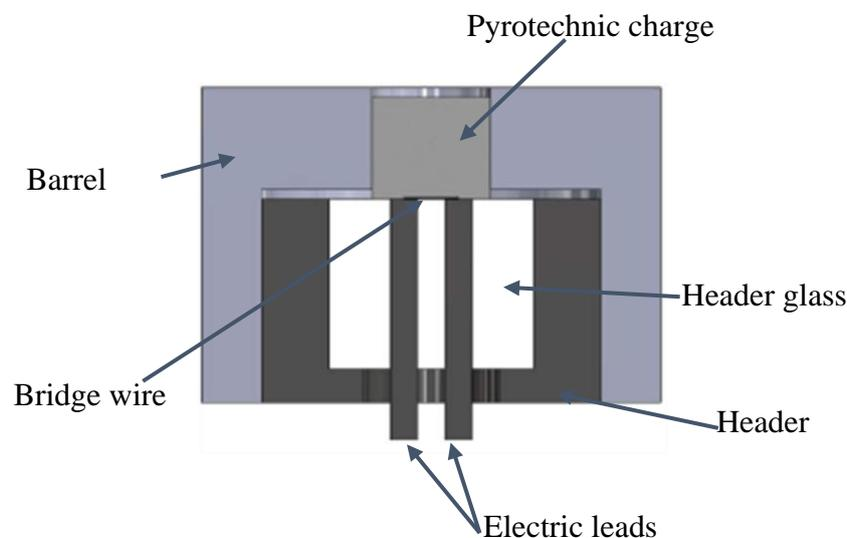
Figure 4.6 Components of hot wire igniter
