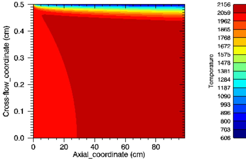
Figure 6. 14 Temperature and velocity distribution in axial direction for inlet flow of BP in non-equilibrium conditions (Axial coordinate vs temperature distribution for 5.00 MPa)
