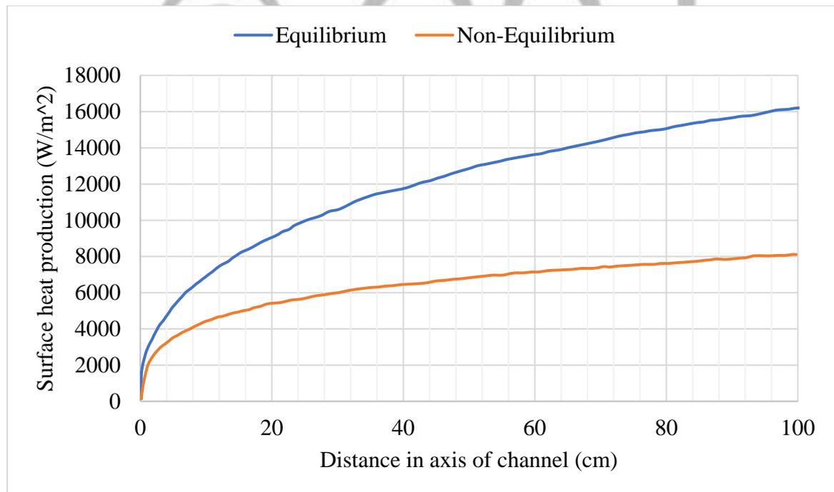
Figure 6.17 Estimated rates of surface heating for inlet flow for an inlet temperature of 2,000<sup>0</sup>K, and inlet pressure 5.00 MPa
