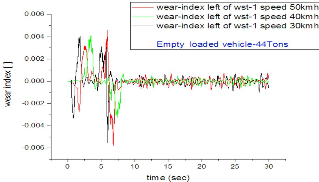
Figure 6 wear index for empty loaded vehicle
