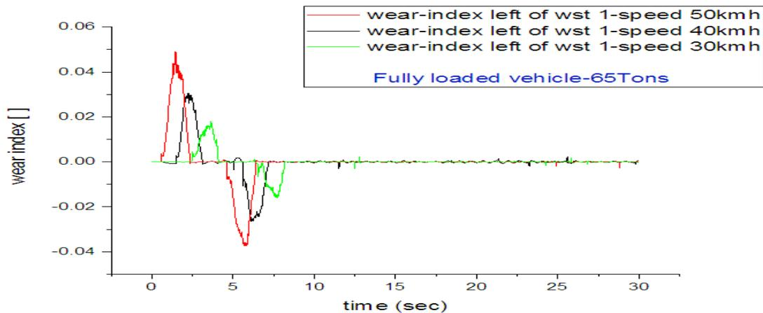
Figure 7 wear index for fully loaded vehicle
