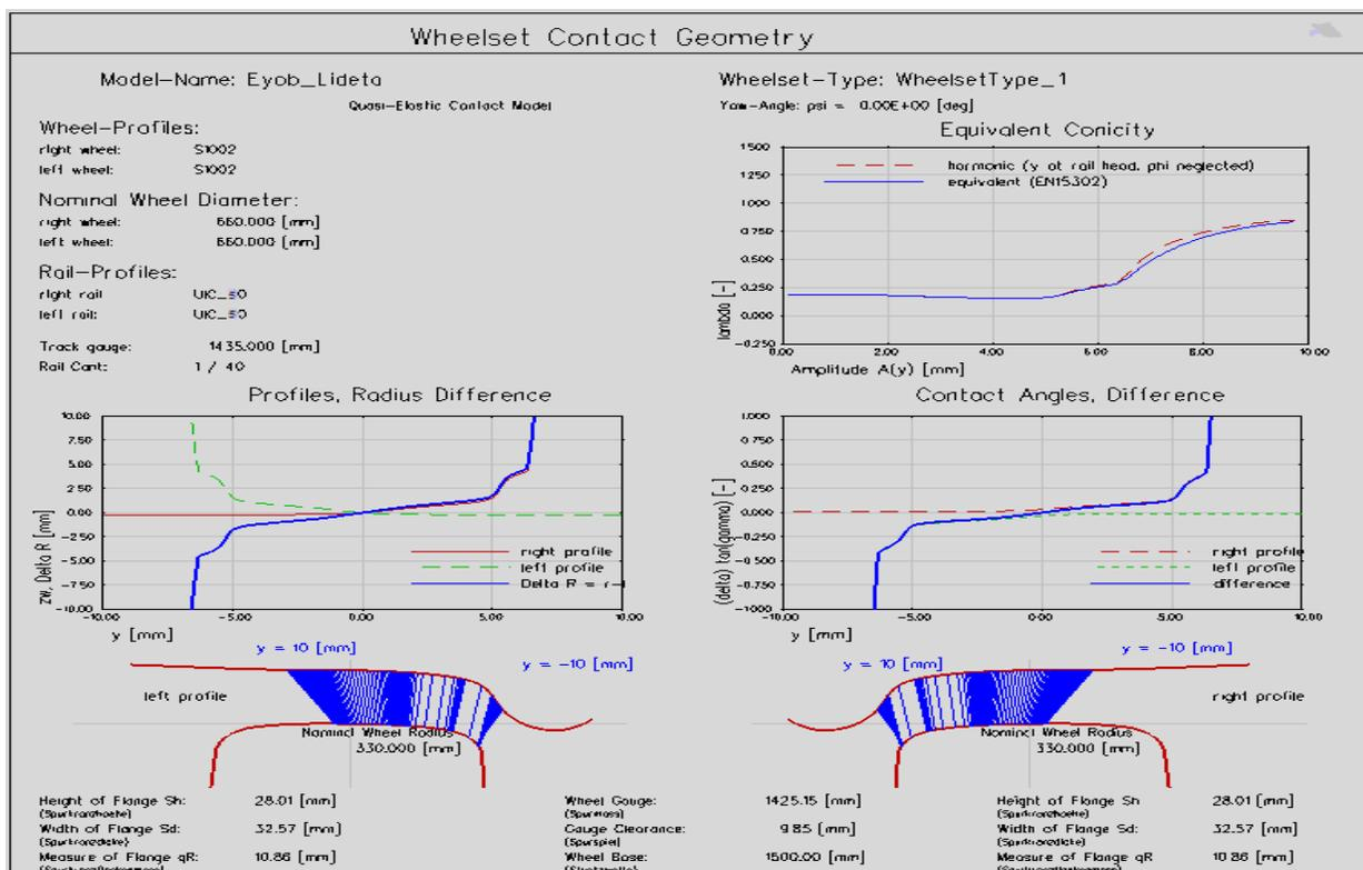
Figure 5 wheel-rail contact
