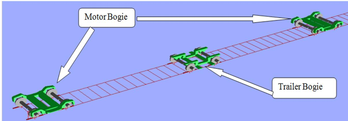
Figure 2 Wheel sets, axle boxes and bogie frames
