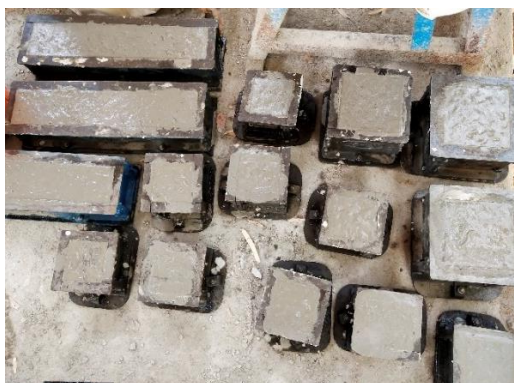
Fig. 3.5 Casting of concrete Specimens
