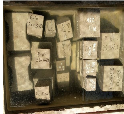
Fig 3.6 Curing of concrete Specimens
