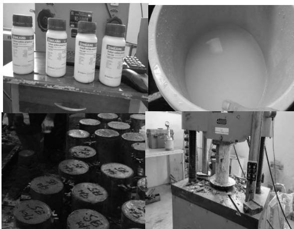
Fig.2. Preparation of 10% Sodium Sulphate Solution, Casting of Cylinders, Curing of Cylinders, and Crushing of Cylinders for Compression strength test.
