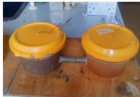
Figure 2.3: Microbial fuel cell containing wastewater from stream
