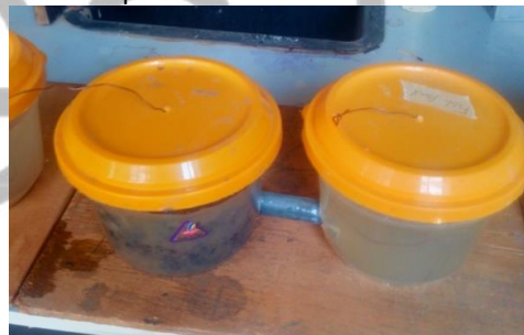
Figure 2.3: Microbial fuel cell containing wastewater from stream
