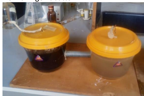
Figure 2.2: Microbial fuel cell constructed with wastewater from fish pond
