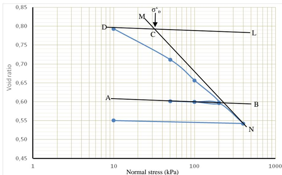
**Figure°4:** Curve of compressibility
