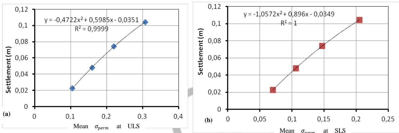
Figure n°6: correlation between settlement under footing and the permissible stress at (a) ULS and (b) SLS
