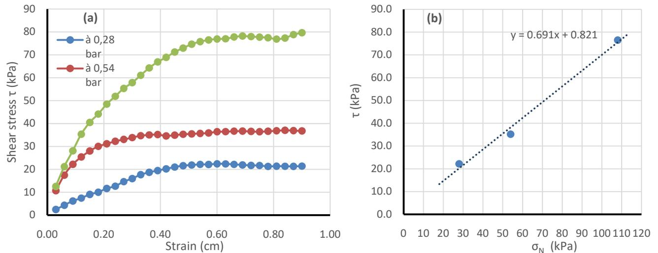
**Figure°3:** Shear test results:(a) Shear stress curve, (b) Shear stress line
