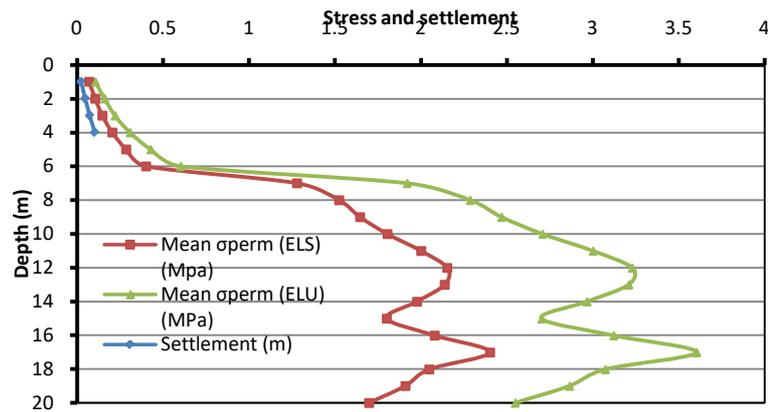
Figure n°5 : Stress and settlement as a function of depth
