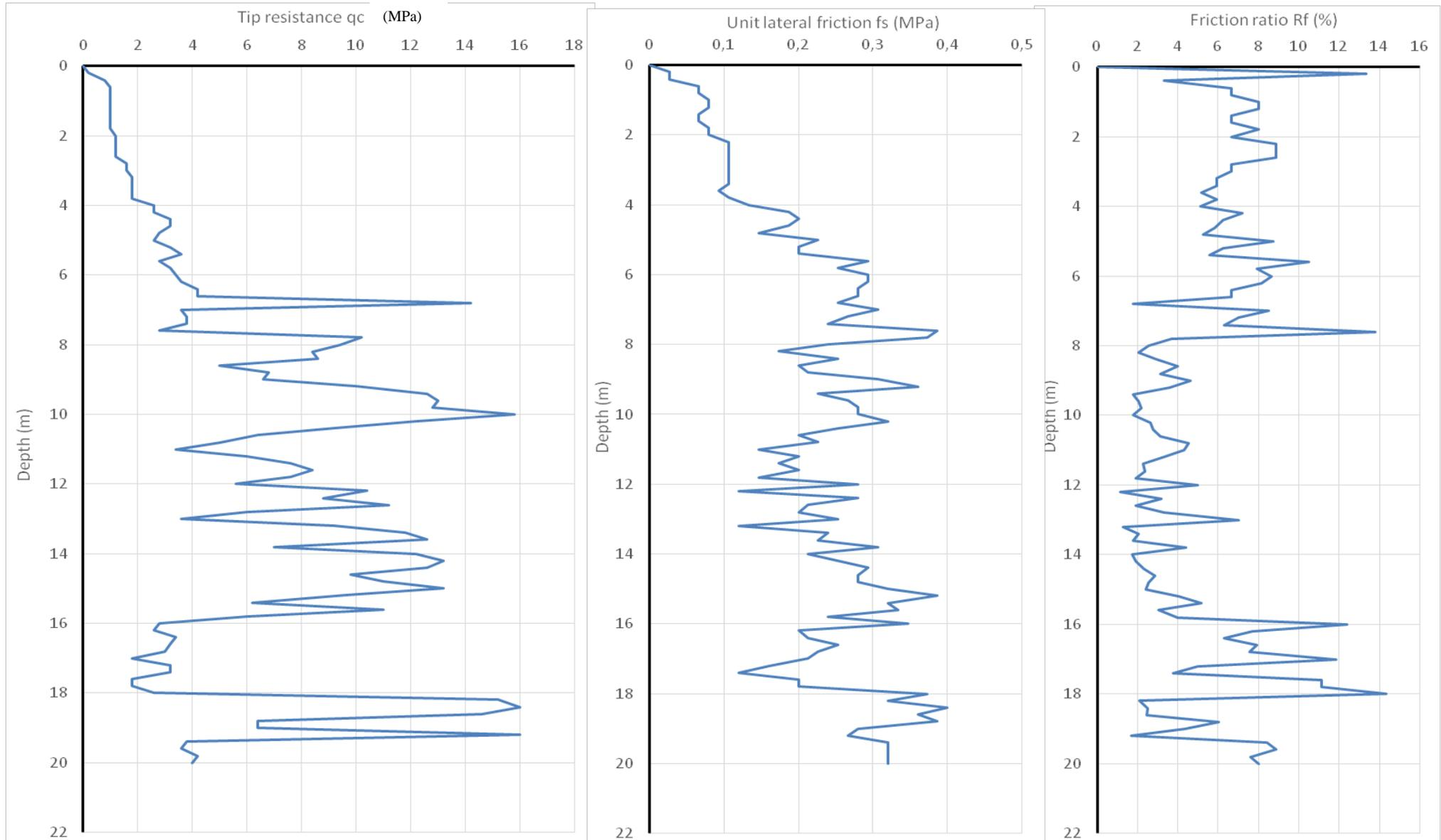
**Figure n°2:** curves of the CPT static penetration test 1
