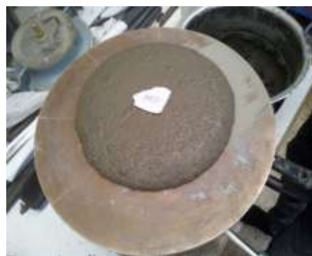
(e) Mortar test for AC-FA 100
