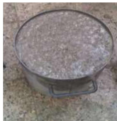
Figure 3.6 : AAC volume remained after casting
