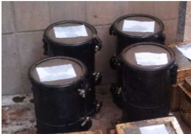
Figure 2.2 Foamed concrete freshly poured into cylinder and cube
