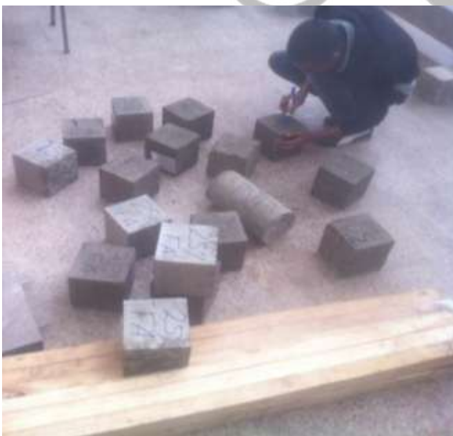
Figure 2.3 Samples after the molds are removed
