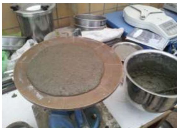
a) Mortar test for CC
