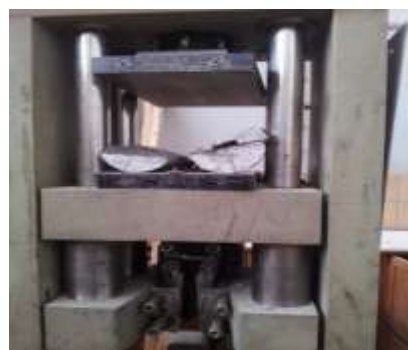
Figure 3.20: splitting tensile test
