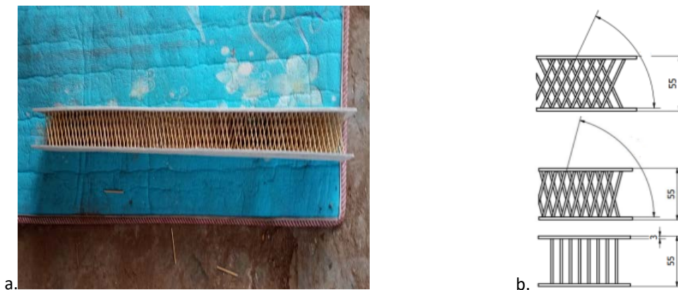
Figure 1a The two sandwich composite skins are connected with bamboo pins, b. The angle of the bamboo pin to the sandwich composite skin: 60^{\circ} , 75^{\circ} dan 90^{\circ}
