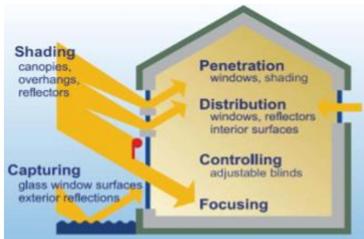
Figure 2.7: Section Showing Natural Lighting
