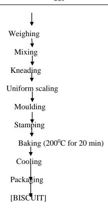
Figure 4: Biscuit Production (Srivastava et al., 2012).
