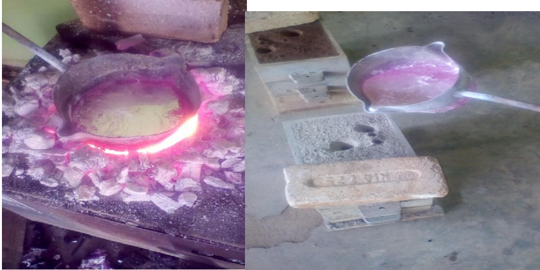
Plate 3 .Aluminum alloy scraps melted in the Furnace.
