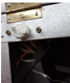
Figure 2.6 Thermostat used in the system
