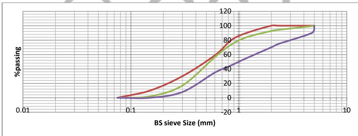
Figure 3.2 Particle Size Distribution for Fine Aggregates in Envelop
