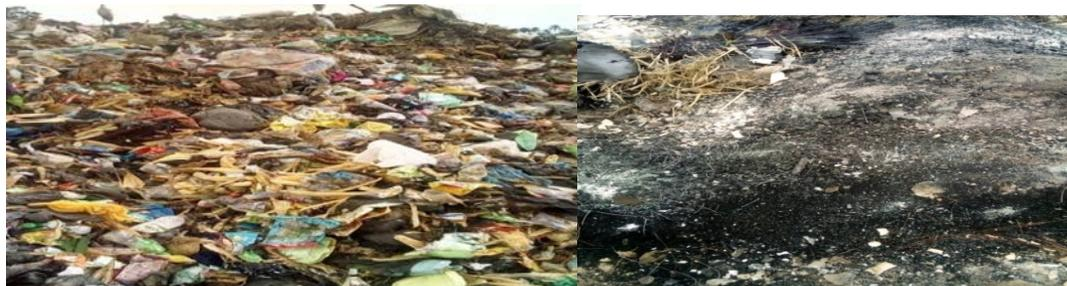
Plate 3.1 (a) MSW before incineration Plate 3.1(b) MSW after incineration.
