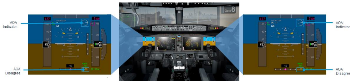
Figure 7: new AOA indicators panel display. Source: Boeing, 2020b.
