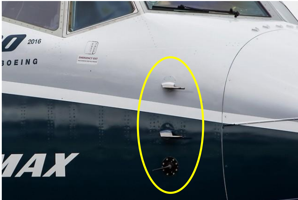
Figure 6: Boeing's 737 MAX Angle of Attack (AOA) sensors. Source: Boeing (2020)
