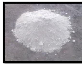
a)Light Grayish white color kaolin b) Plasticity of kaolin surfaces c)Powdered Kaolin samples
