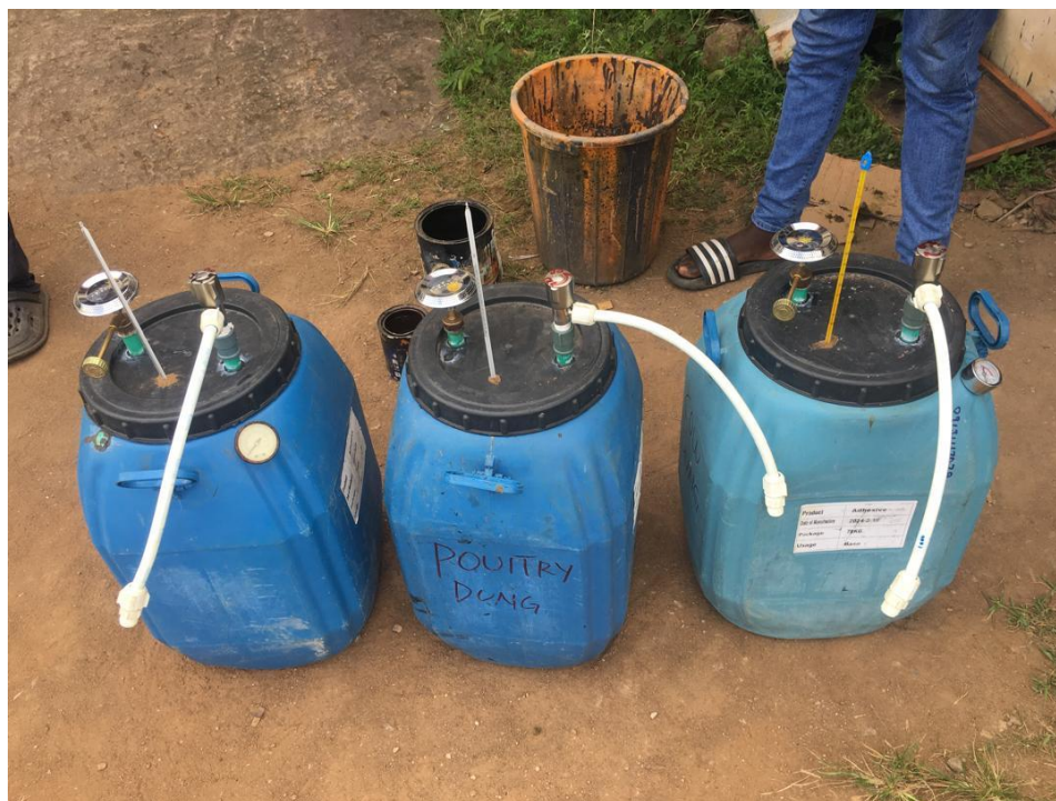
Plate 1. Installation of pressure gauges, gas valves and thermometers on the digester's cover
