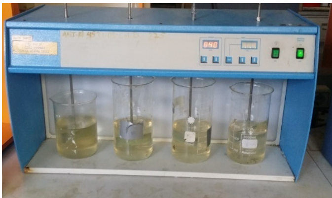
Figure 3.4 Jar test to determine hydrated aluminum sulfate dosage
