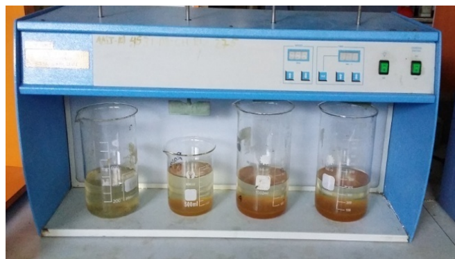
Figure 3.2 Jar test to determine ferric chloride dosage
