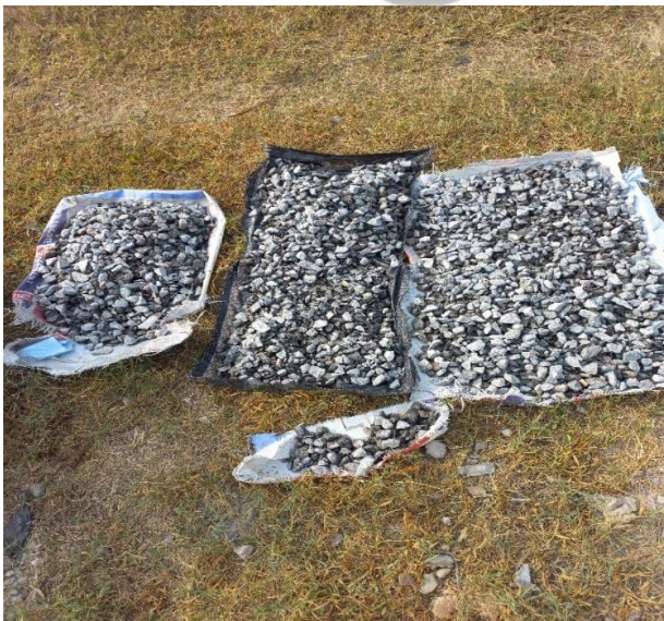
Fig 4.1: Drying of coarse aggregate after being washed with potable water
