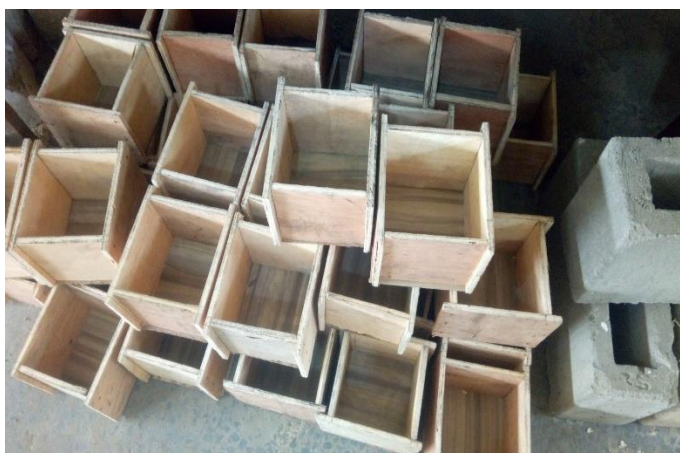
Fig 4.3: Wooden moulds for casting all samples
