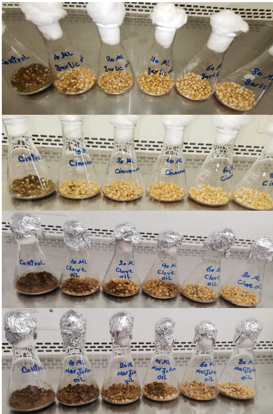
Figure(6): Effect of different concentrations of (a) garlic,(b) cinnamon, (c) clove and(d) marjoram essential oils in controlling OTA production in corn grains.
