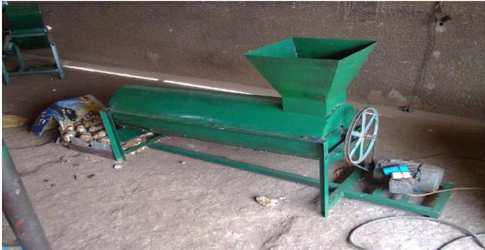
Fig 3. Sweet potato peeling machine with fixed components
