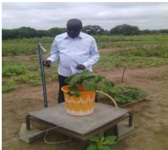
Plate 1: A typical set up of the mini-lysimeter.
