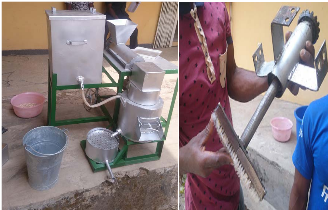
Figure 3. NCAM developed wet cowpea dehuller and the incorporated brush for separation cleaning of the dehulled cowpea.
