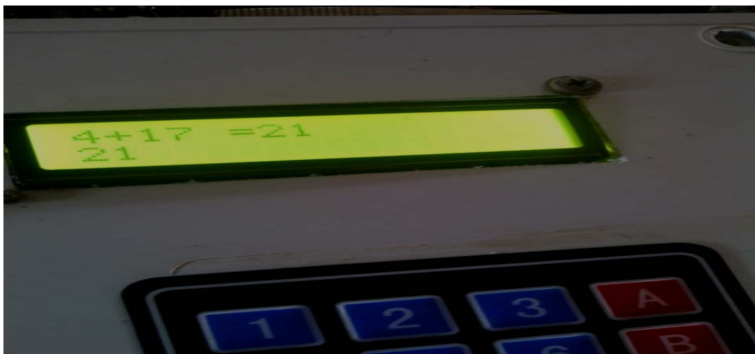
Figure 4.4: Showing the addition operation of the Keypad of the Calculator
