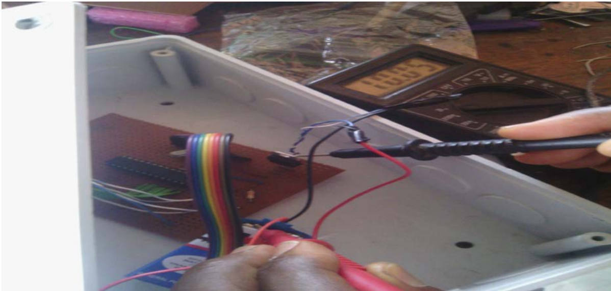
Figure 4.1: Showing the continuity test of the design circuit with multimeter
