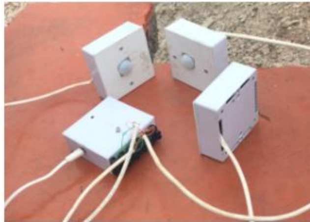
Figure 6: Constructed Intruder Detector System
