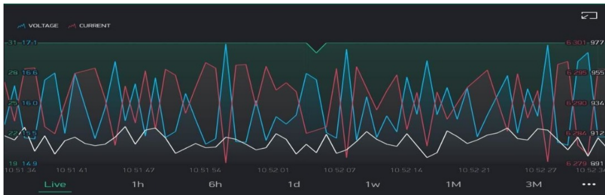
Figure 5: User Interface showing Graph of Voltage and Current against Time
