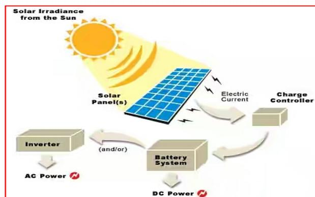
Figure 2-2 Schematic drawing of stand-alone PV system
