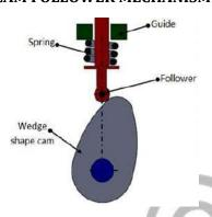
This cam follower feeder mechanism convers rotary motion into linear motion.
