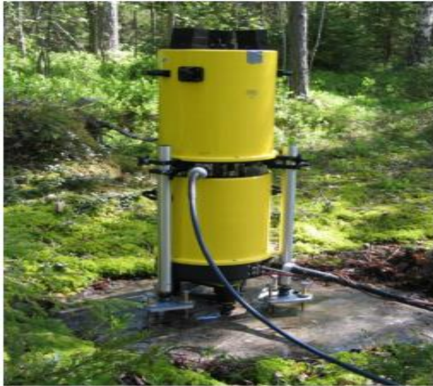
Figure 1. A10-020 absolute gravimeter setup on a bedrock station in Sweden
