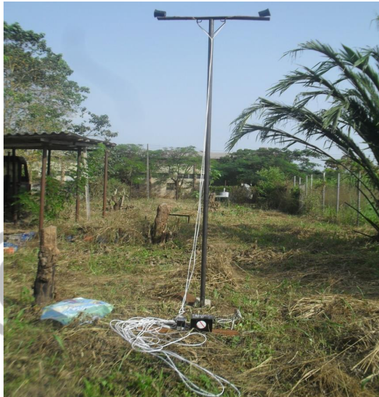
Fig. 3: The assembled bird scarer
