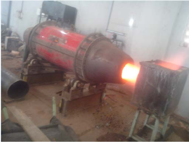
Plate 1: Rotary furnace at a preheating stage.
