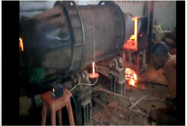
Plate 2: Tapping of molten cast iron.
