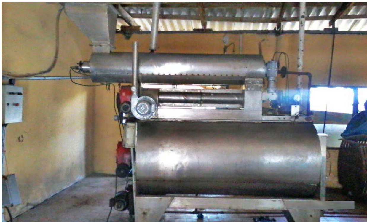
Plate 1: Compact Fishmeal Processing Plant (Denmark, type FR100)
