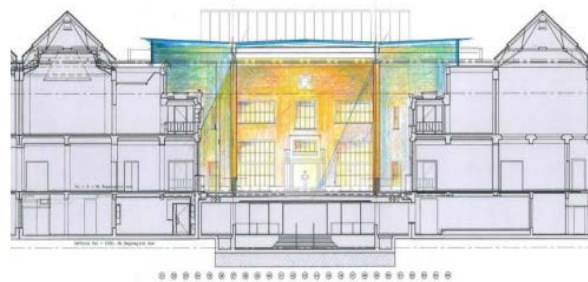
Figure 4.13- Section of the museum, the design of top-lighting apertures in the top galleries and suspended elements inside the roof structure is visible
