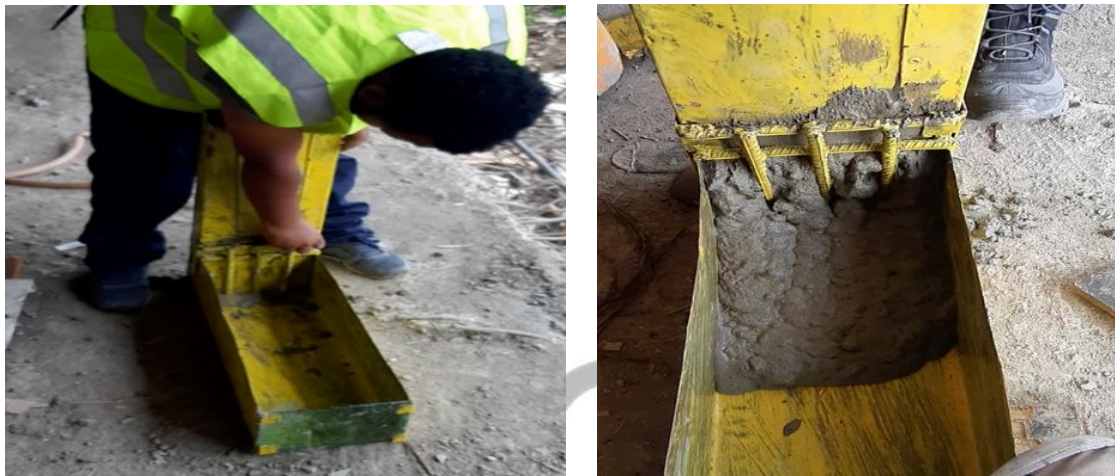
Figure 2.5: L-box test of self-compacting concrete.
