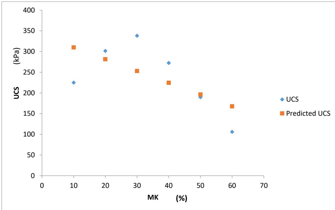
**Figure 3.4: Unconfirmed Compressive Strength against Metakaolin (MK line fit Plot)**
