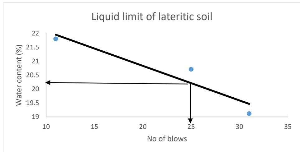
**Figure 3.1: Liquid limit of natural lateritic soil**
