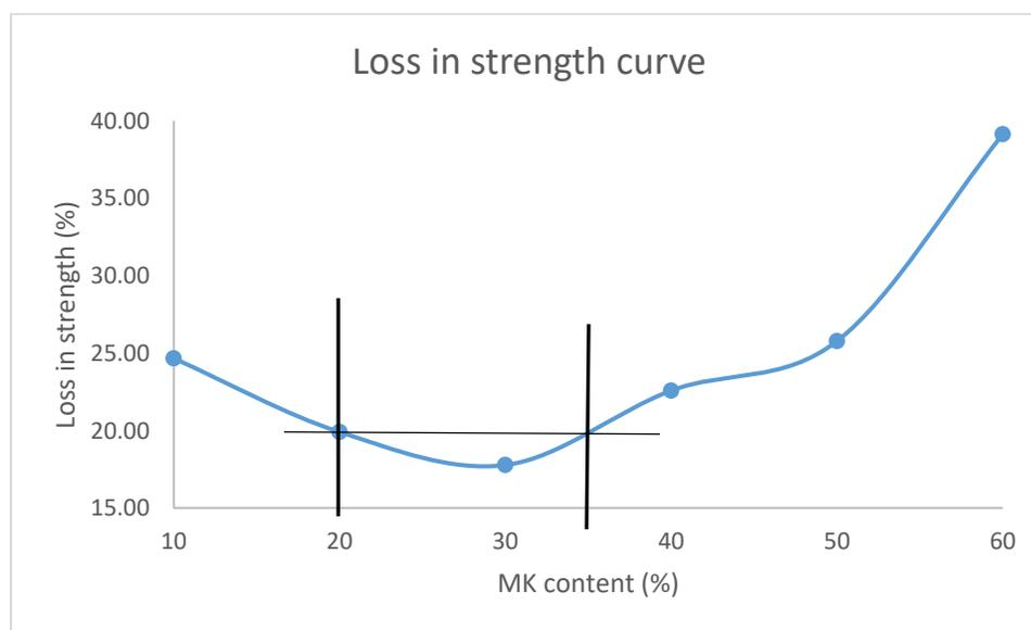
**Figure 3.5: Loss in strength Vs MK content**
