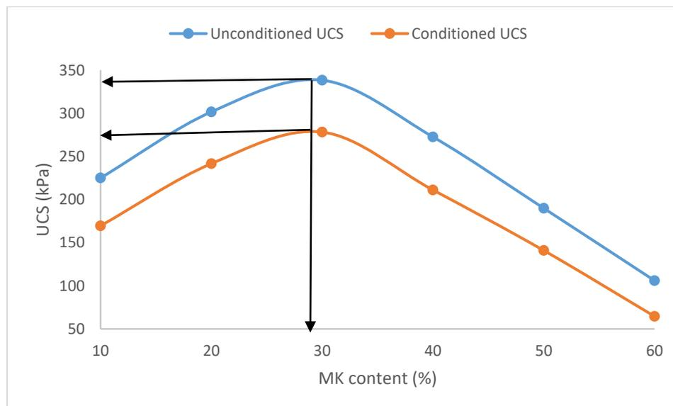
**Figure 4. 3 UCS Vs MK content (Unconditioned and Conditioned MK-lateritic soil)**
