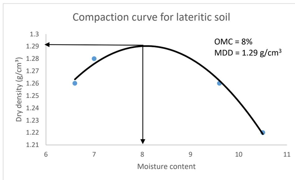
**Figure 3. 2 Dry density Vs moisture content of natural lateritic soil**
