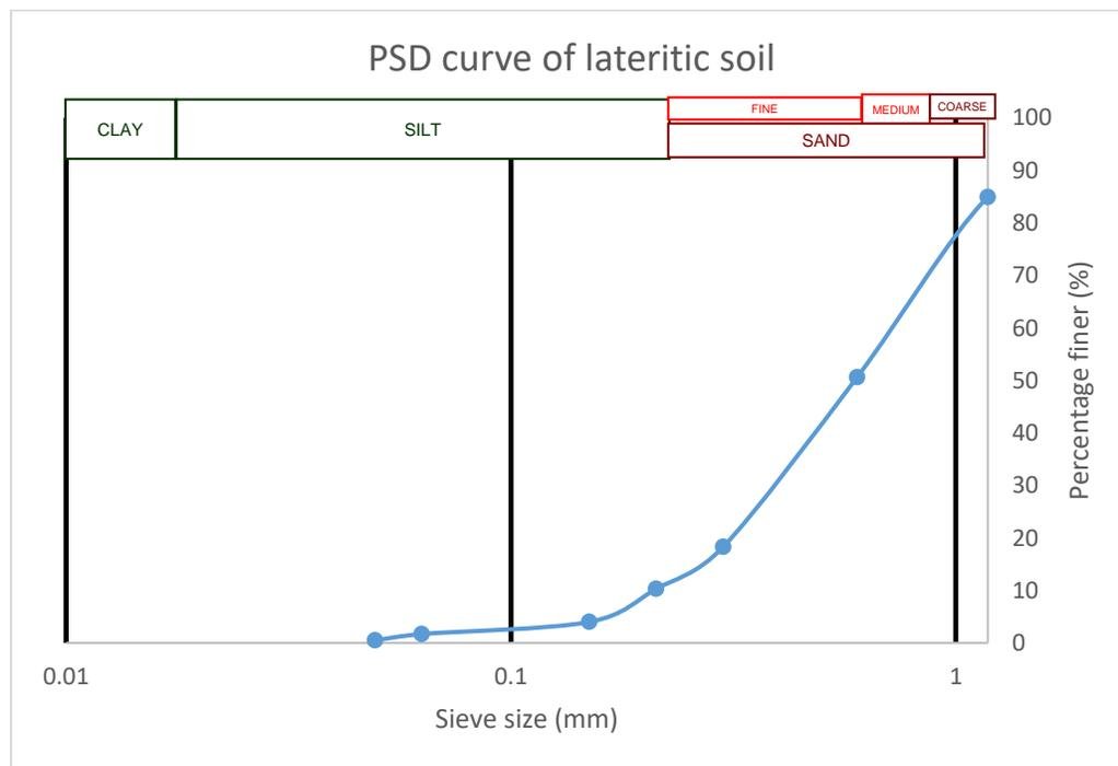
Figure 3. 1 Particle Size Distribution Curve of natural lateritic soil
