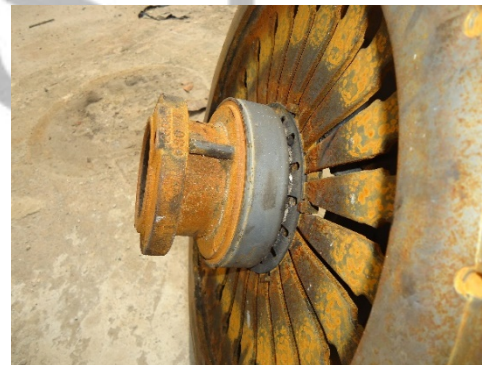
Fig.2: Clutch plate of an Actross Truck.
