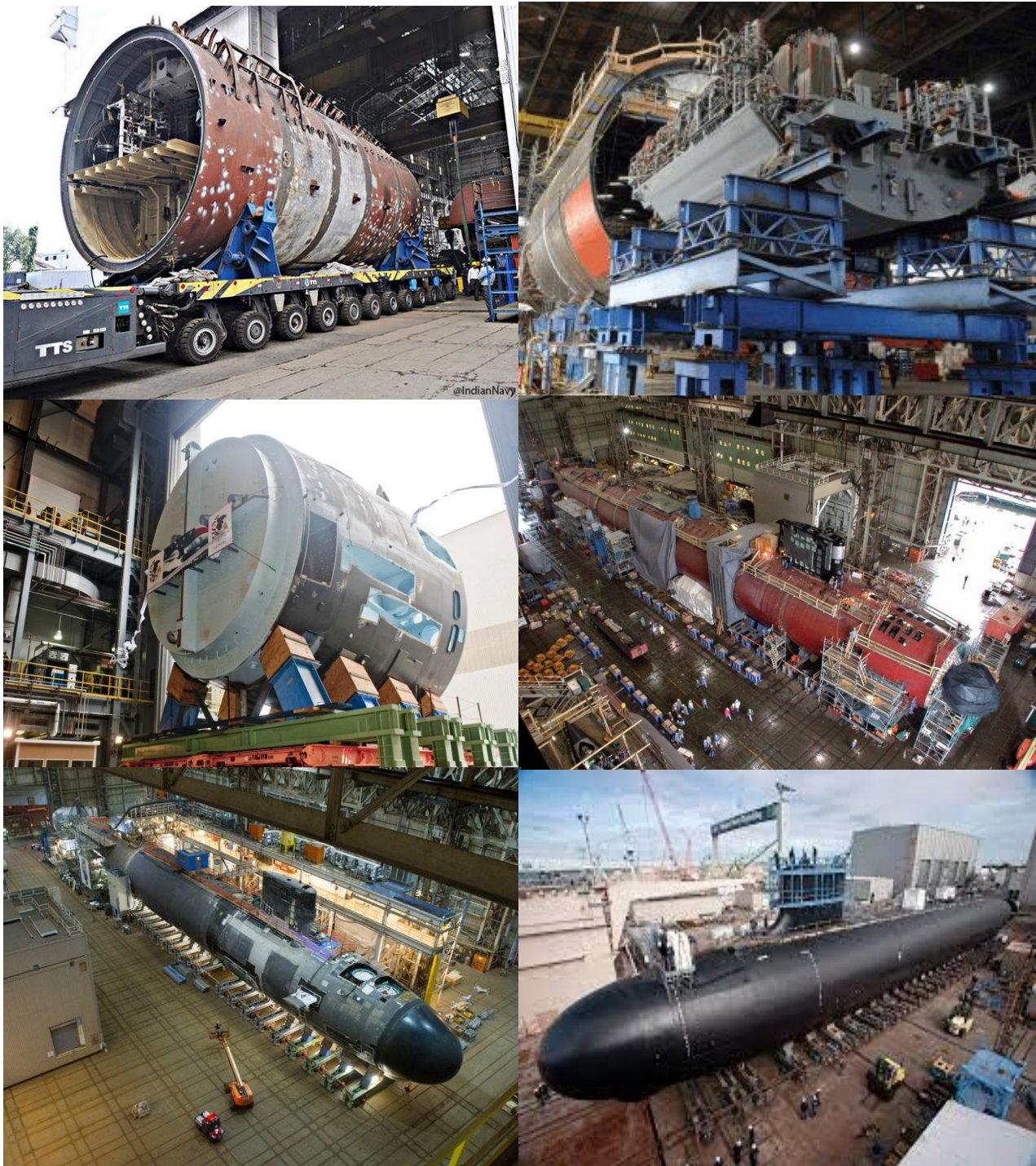
Figure 13: Module Construction of Submarine (Virginia-class Nuclear Power submarine of the US Navy) 20
