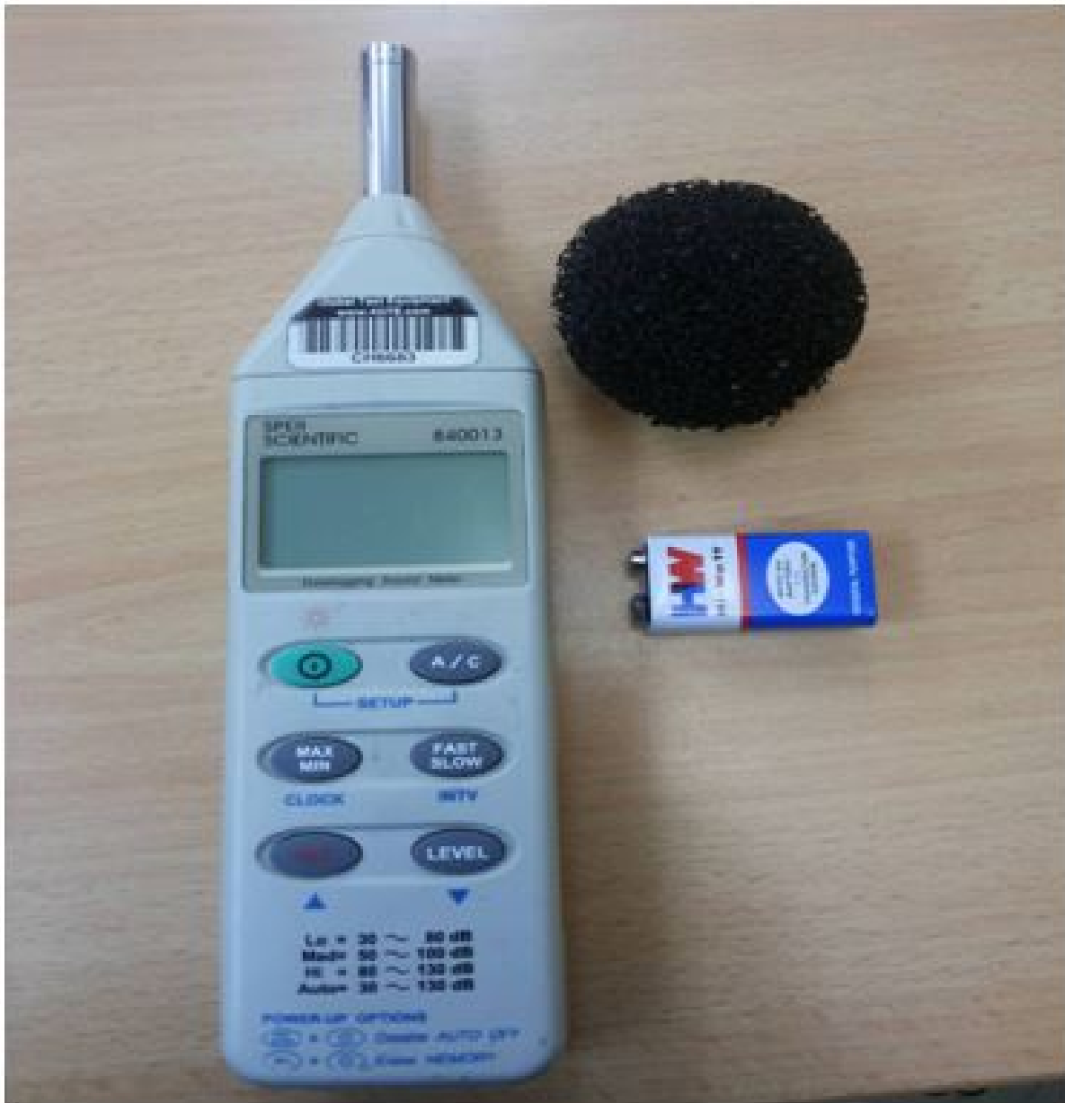
Plate 1: Sound Level Meter - Model 840013, Decibel (Db) low range (dB) 30 / high range (dB) 130, Resolution (dB) 0.1, Accuracy \pm 1.5 dB, Response: fast (125 millisecond), slow (1 second) and Battery Type: 9v battery (1).
