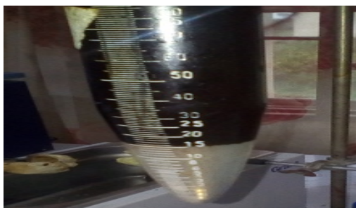
Figure 5. Clear water separated with sharp oil-water interface
