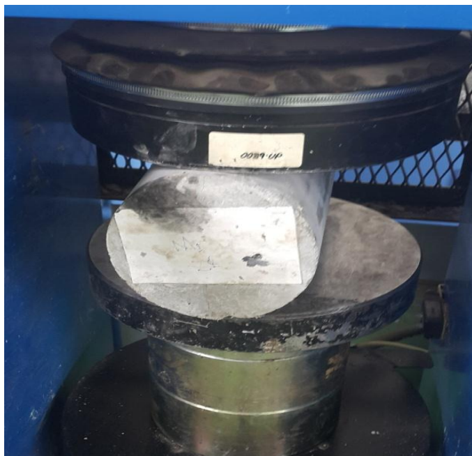
Figure3: Compressive and split tensile strength testing machine & cube and cylinder under loading.
