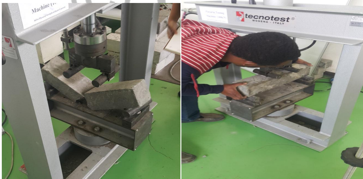
Figure4: Flexural strength testing machine and beam under third-point loading.
