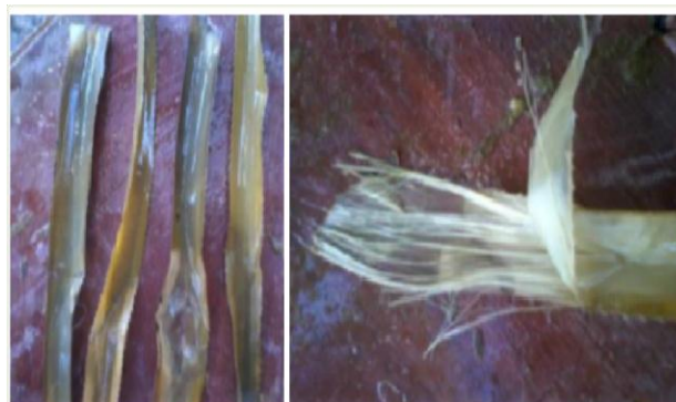
Figure 3: Pineapple leaf fiber extraction by retting methods
