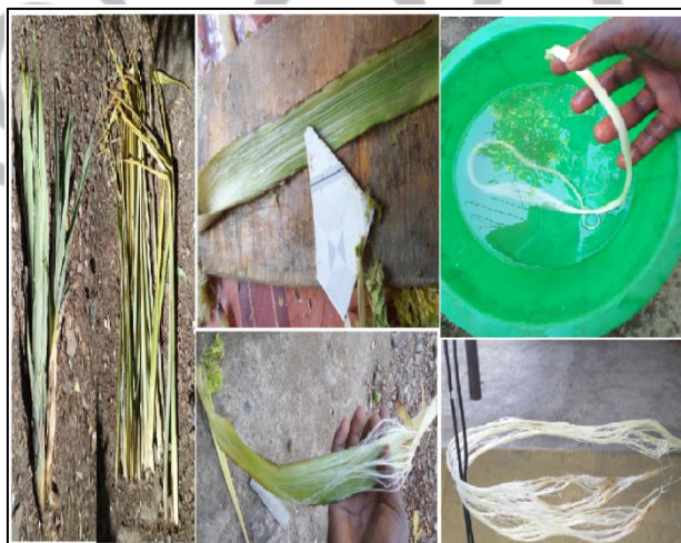
Figure 2: Pineapple leaf fiber extraction by scrapping method
