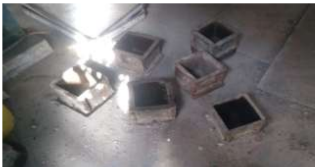
Figure 1: Cubic mould (15cm ×15cm ×15cm)
