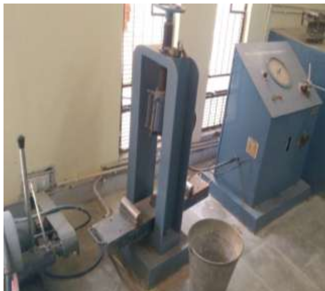
Figure 11: Flexural testing machine
