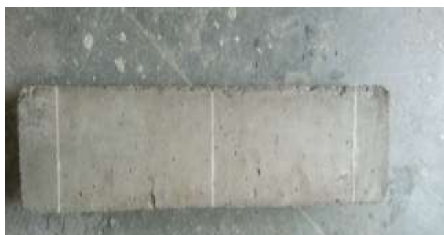
Figure 12: prepared beam sample for flexural test
