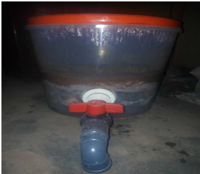
The constructed sand filter
