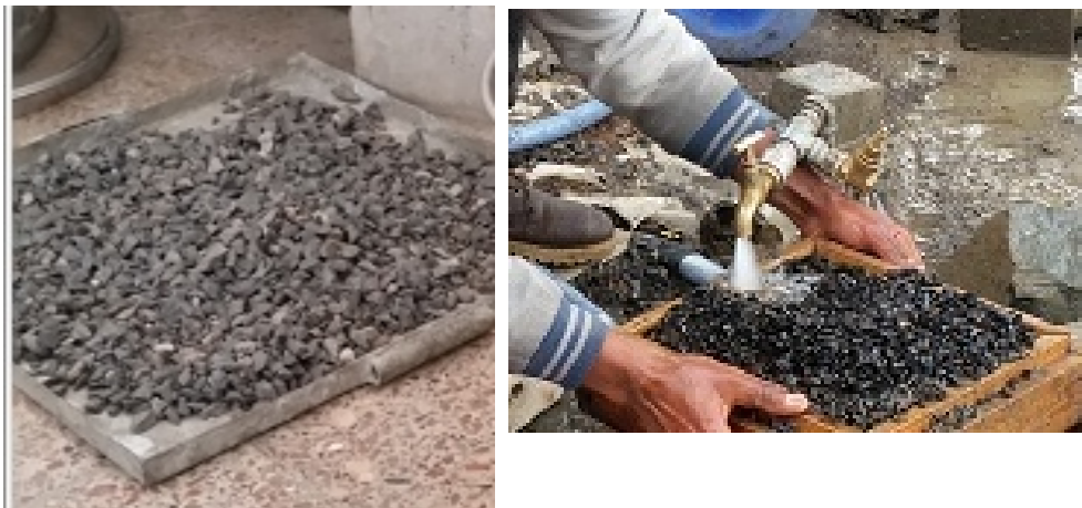
Fig. 2.2 Washed coarse aggregate used for the study (left), washing aggregate (right)
