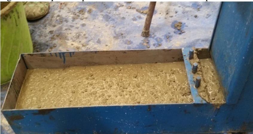
Fig. 4.2 L- Box flow of SCC without cement replacement
