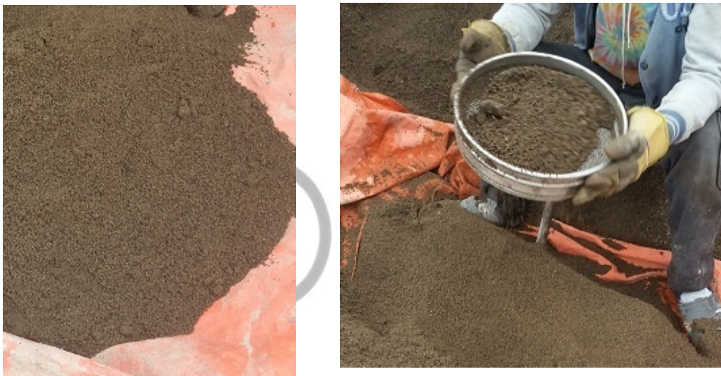
Fig. 2.3 Fine aggregate (sand) (left) and sieving for fine aggregate (right)
