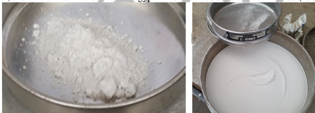
Fig. 2.1 SEDE gypsum powder on a pan (left) and Determination of gypsum fineness (right)
