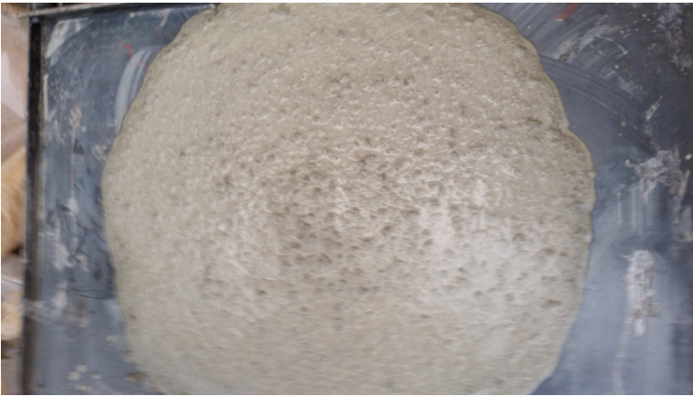
Fig. 4.1 Slump flow spread of SCC without cement replacement
